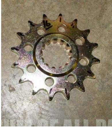
Figure 6.2 COUNT THE TEETH! Make sure it matches the # for your kit.
