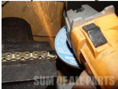
Figure 7.86 grind off heads
