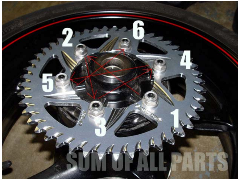
Figure 6.15 tighten bolts in a star-cross pattern making sure to not over tighten.
